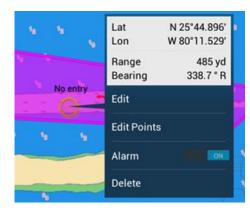
When the own ship approaches the area within 300 yd, Near Alarm will be generated. While the alarm bar shows the message [Near Alarm Zone: No entry], the data box shows the distance to the area with an alert icon [!] in yellow.
